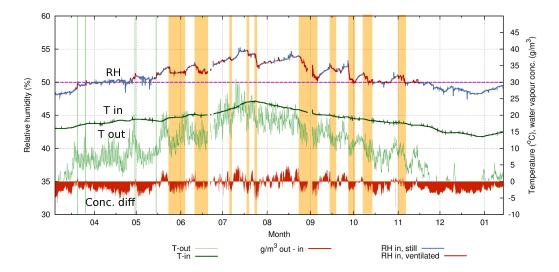
Figure 5: The year 2010 in the archive. The shaded vertical strips indicate periods when outside air was pumped in to raise the air exchange rate from 0.1 per hour to 0.5 per hour. The shaded strips correlate with the difference in water vapour content between the outside and the archive air. The dashed horizontal line marks the target RH.
