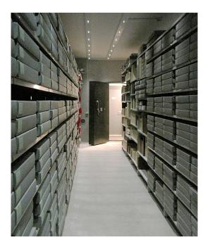
Figure 1: A view of the interior of the archive. It measures  $10 \times 4 \times 3$  m high. The lobby is visible beyond the armoured and insulated door. The duct for pumped outside air is just visible above and to the left of the door.
