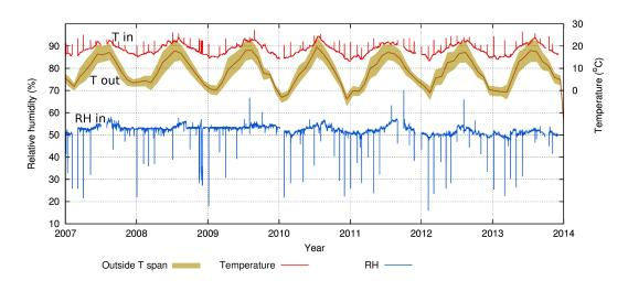
Figure 4: A record of the archive climate over seven years, compared with the monthly average outside temperature and temperature span. The spikes show the climate in the conservator's office when the logger was retrieved to extract its data.
