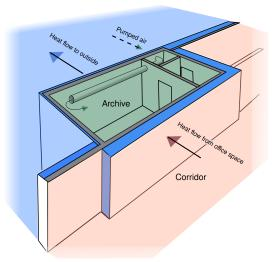
Figure 3: A perspective sketch showing how the archive temperature is set by the competing heat flows through the interior walls and the exterior walls. The RH is fine-tuned by pumping in air when by chance the outside air has suitable water vapour content.
